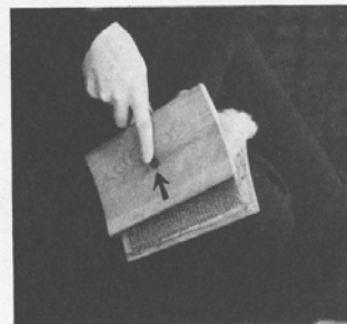
5. Bring handles together to roll off the wool.
