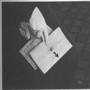
4. Reverse direction of carding for persistent noils; continue carding.
